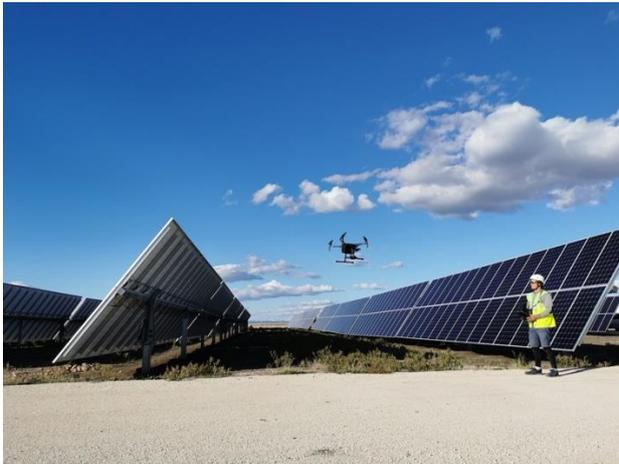
*Caption: Volateq's solution enables drone-based health checks of solar fields by intelligent image analysis*
